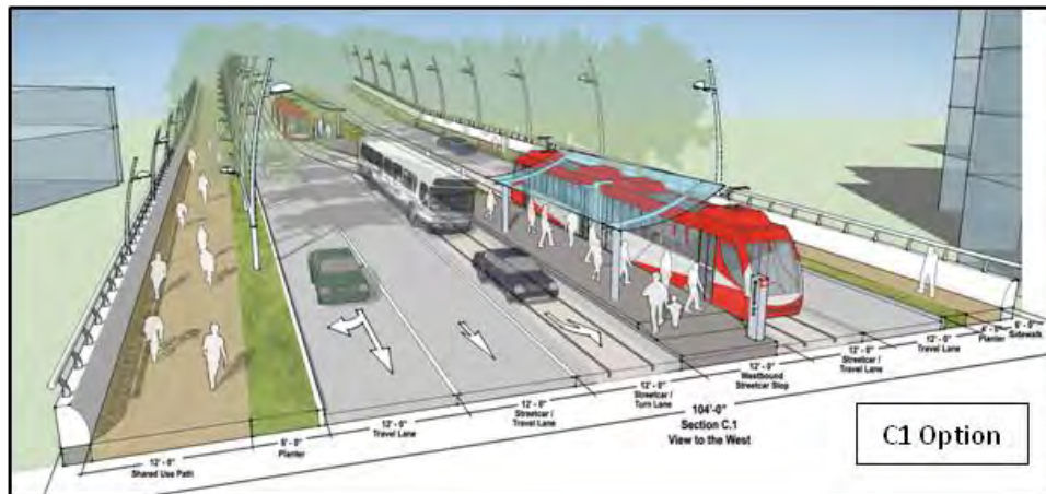
Figure 7: Benning Road Viaduct Cross Section Options
