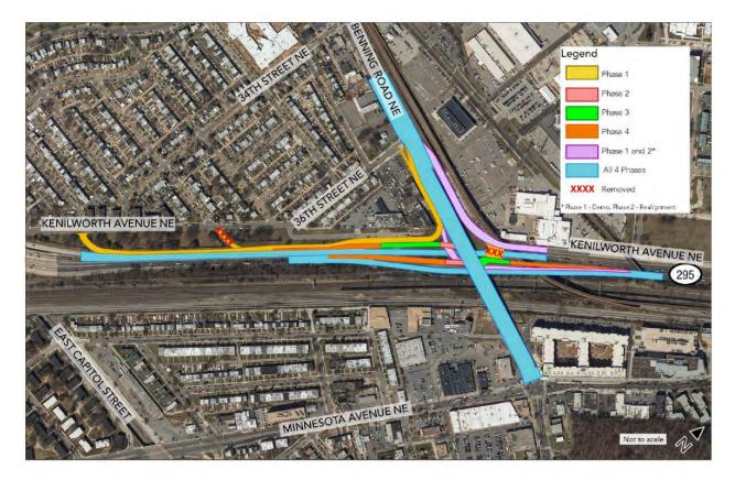
Figure D-2. DC 295 - Benning Road Interchange Improvements Phasing Diagram
